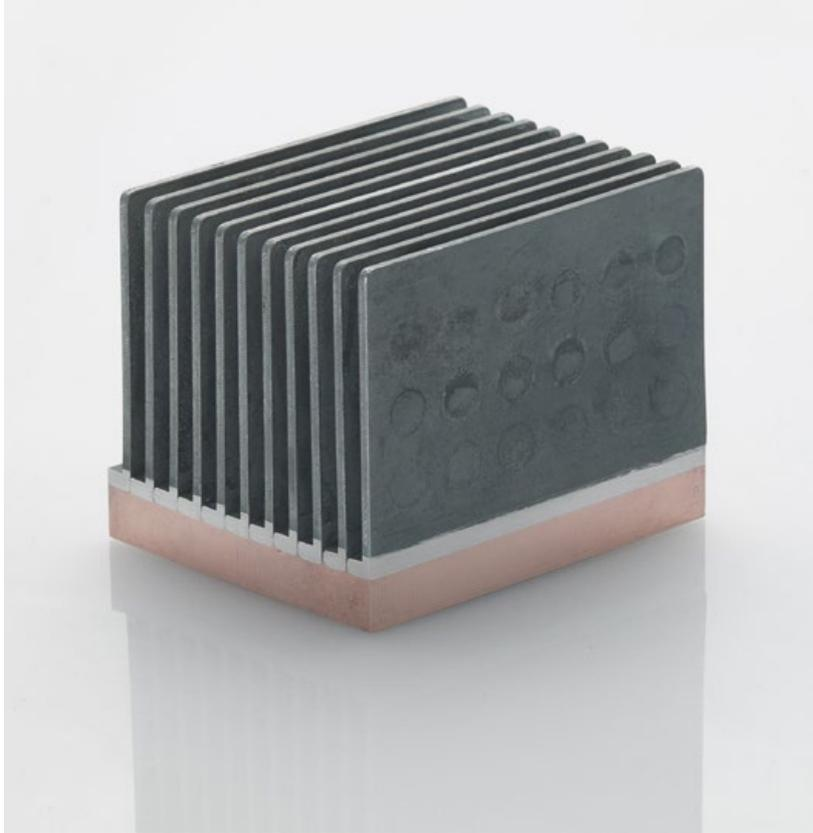
Fig. 12 A multi-material heat sink created by depositing copper powder onto aluminium fins to create a heat sink that is high performance, low weight and inexpensive to produce. This 200 g part weight took two minutes to produce
